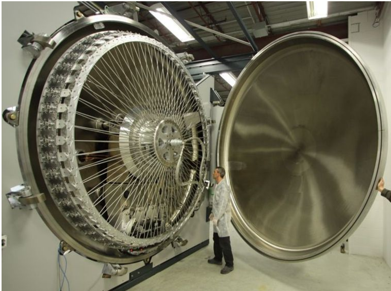
Figure 9 Photograph of the wafer drum
